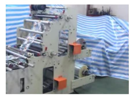
Figure 3: Sleeve cutting machine. url: https://www.youtube.com/watch?v=kbQ-Q8TCvS0
