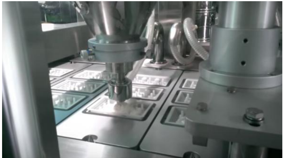
Figure 7: One step in the process in producing the product. The Vectorite powder is being placed into the Vectorpak™ (Bee Vectoring Technology, 2015).
