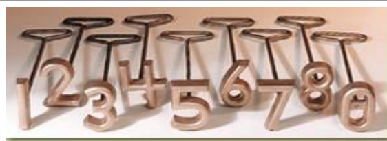
Example of copper brands used (source: http://stockyardsupply.com/wp-content/uploads/2013/08/FreezeBrand.jpg )
